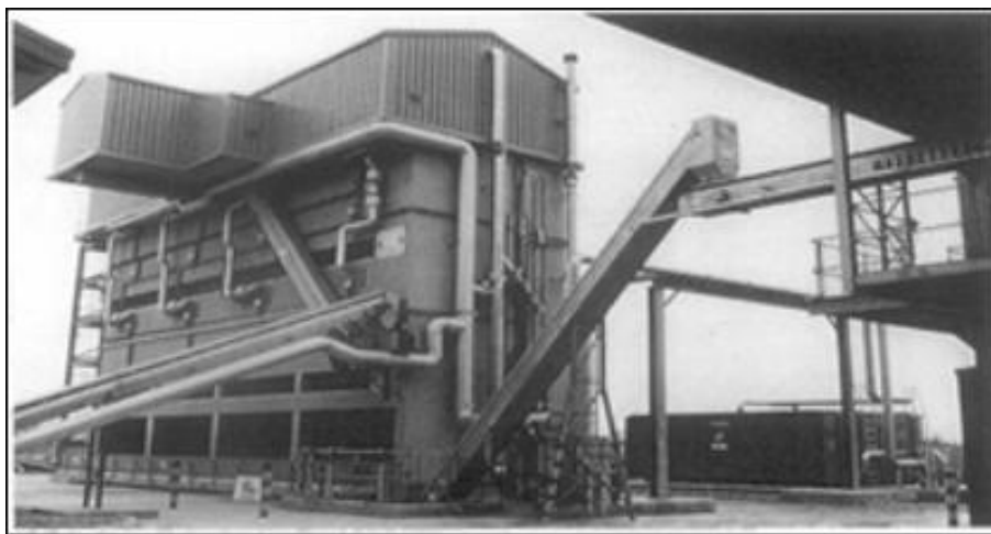
Figura 9: Sistem de reactor vertical (tip siloz)
